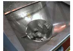
Feed hopper directs material down into the crusher's fixed cast cutters and rotating arm.
