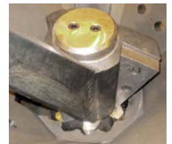
Fixed and rotating rings are used in final crushing stage
