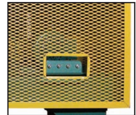
Lubrication points are centrally located for easy access and maintenance.
