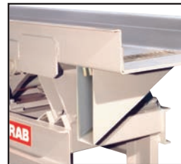
Screening and sorting configuration with side discharge chute.
